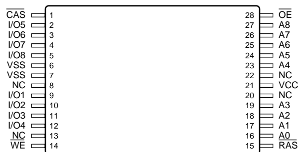
28 Lead TSOP-I PIN CONFIGURATION Top View
