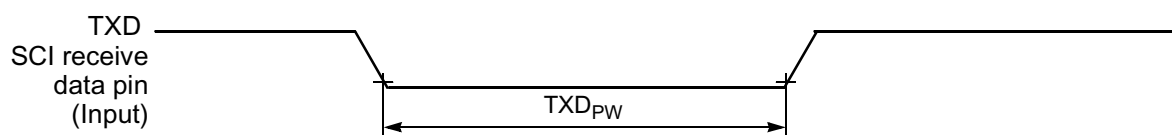
Figure 10-17 TXD Pulse Width
