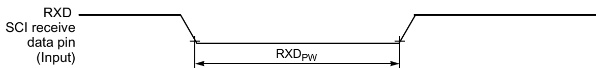
Figure 10-16 RXD Pulse Width
