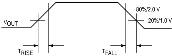
Figure 3. WAVEFORMS: Rise and Fall Times
