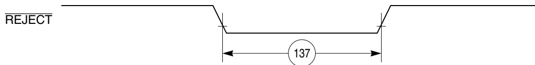
Figure 64. CAM Interface REJECT Timing Diagram
