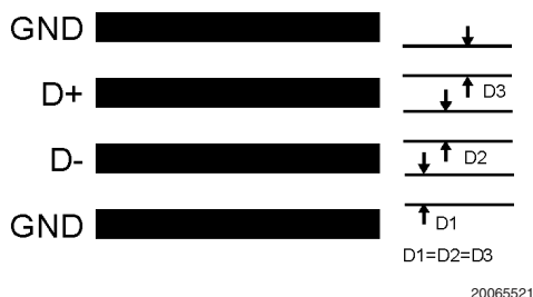
FIGURE 11. Ideal Diode Trace Layout
