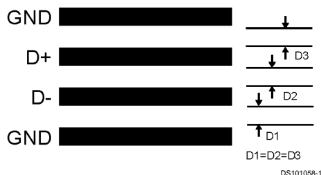
FIGURE 10. Ideal Diode Trace Layout
