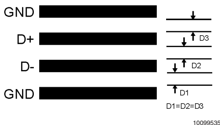
FIGURE 9. Recommended Diode Trace Layout
