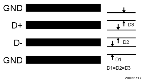
FIGURE 15. Ideal Diode Trace Layout
