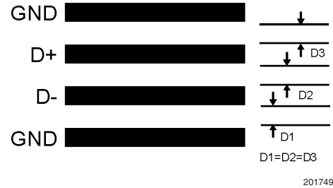
FIGURE 8. Ideal Diode Trace Layout
