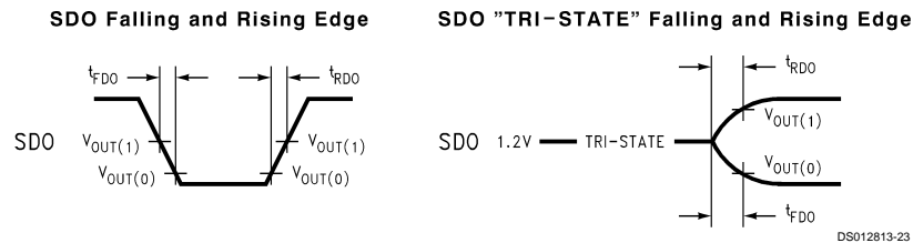
FIGURE 15. SDO Timing
