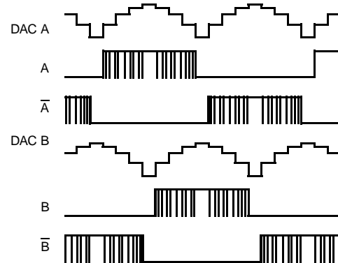
Figure 19: Stepper Motor Waveform - LM9830 Signals
