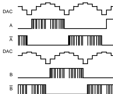
Figure 11: Stepper Motor Waveform - LM9832 Signals
