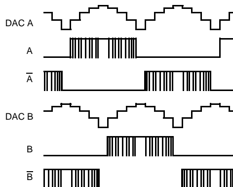
Figure 11: Stepper Motor Waveform - LM9833 Signals
