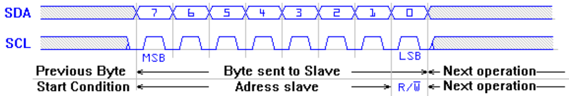
Figure 6. Basic I2C Timings
