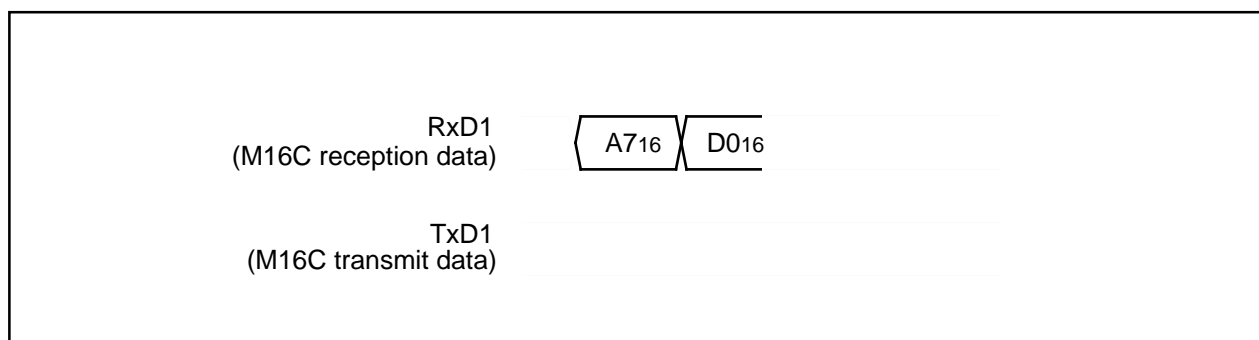
Figure 1.25.27. Timing for erasing all unlocked blocks
