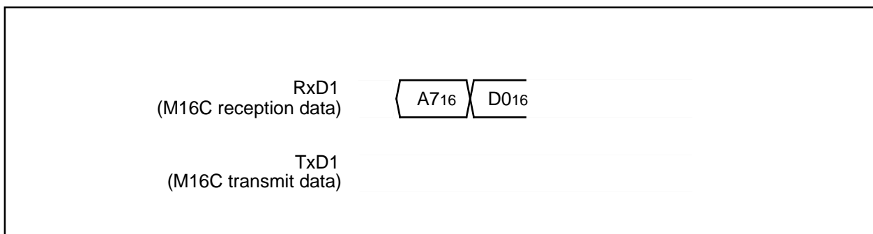
Figure 1.32.27. Timing for erasing all unlocked blocks
