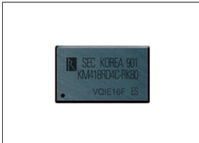
Figure 1: Direct RDRAM CSP Package
