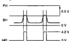
Figure 9. High-frequency level comparator signal
