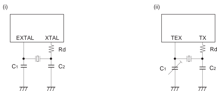
Fig. 13. Recommended oscillation circuit
