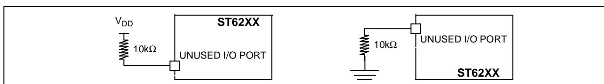
Figure 62. Two typical Applications with unused I/O Pin
