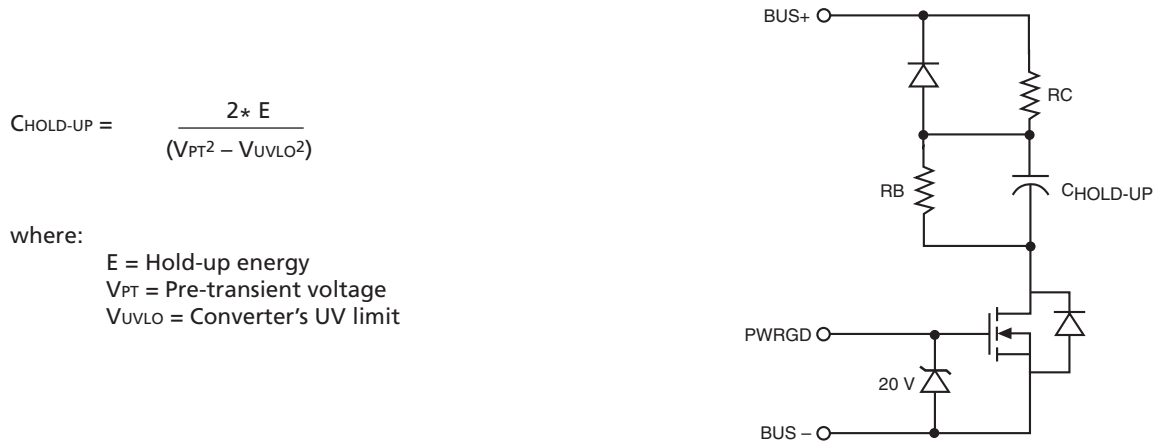
Figure 9c – Powergood controlled, auxiliary bulk storage capacitor charging circuit.
